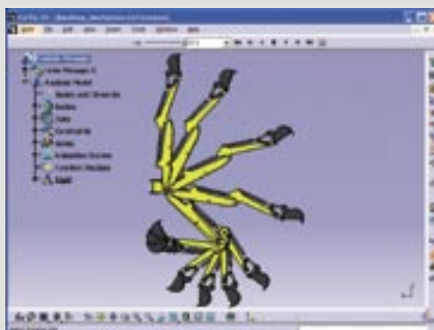
Create motion envelopes of the moving mechanism.
