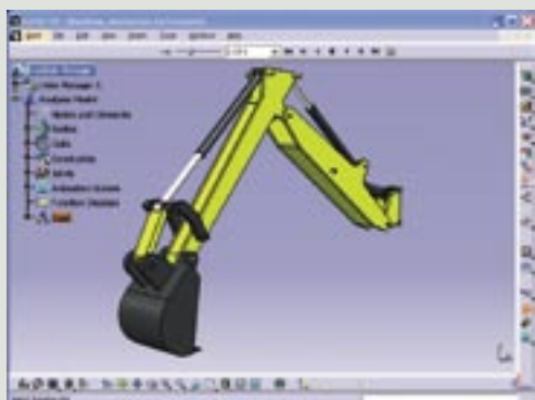
Extend CATIA V5 assemblies with joints, forces, motion drivers and gravity.
